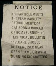
Furniture foam to withstand a small open flame for 12 seconds
